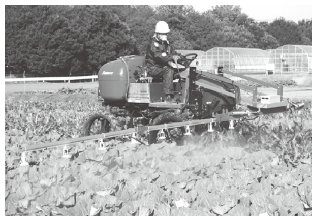
Fig. 3. Boom-type electrostatic sprayer 7.4 kW gasoline engine, Nozzle span: 300 mm, Spraying width: 15 m, Nozzle operating pressure: 1.5 MPa, Nozzle flow rate: 1.7 L/min., Hollow-cone spray: VMD 112 \mu m
