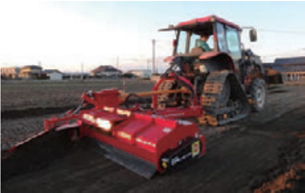
Fig. 10. Modified type of embankment topsoil removal machine
