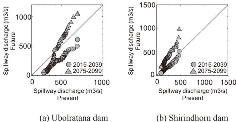
Fig. 14. Changes in daily spillway discharge at the (a) Ubolratana and (b) Shirindhorn dams
