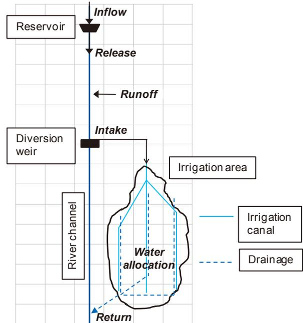
**Fig. 3. Conceptual diagram of water management in an extensive and well-developed irrigation system with a reservoir**
