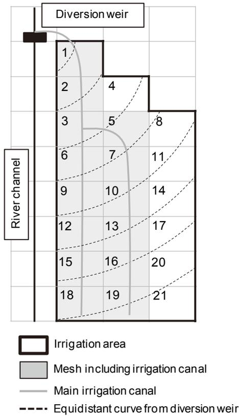
**Fig. 5. Conceptual diagram of a water allocation and management model**
