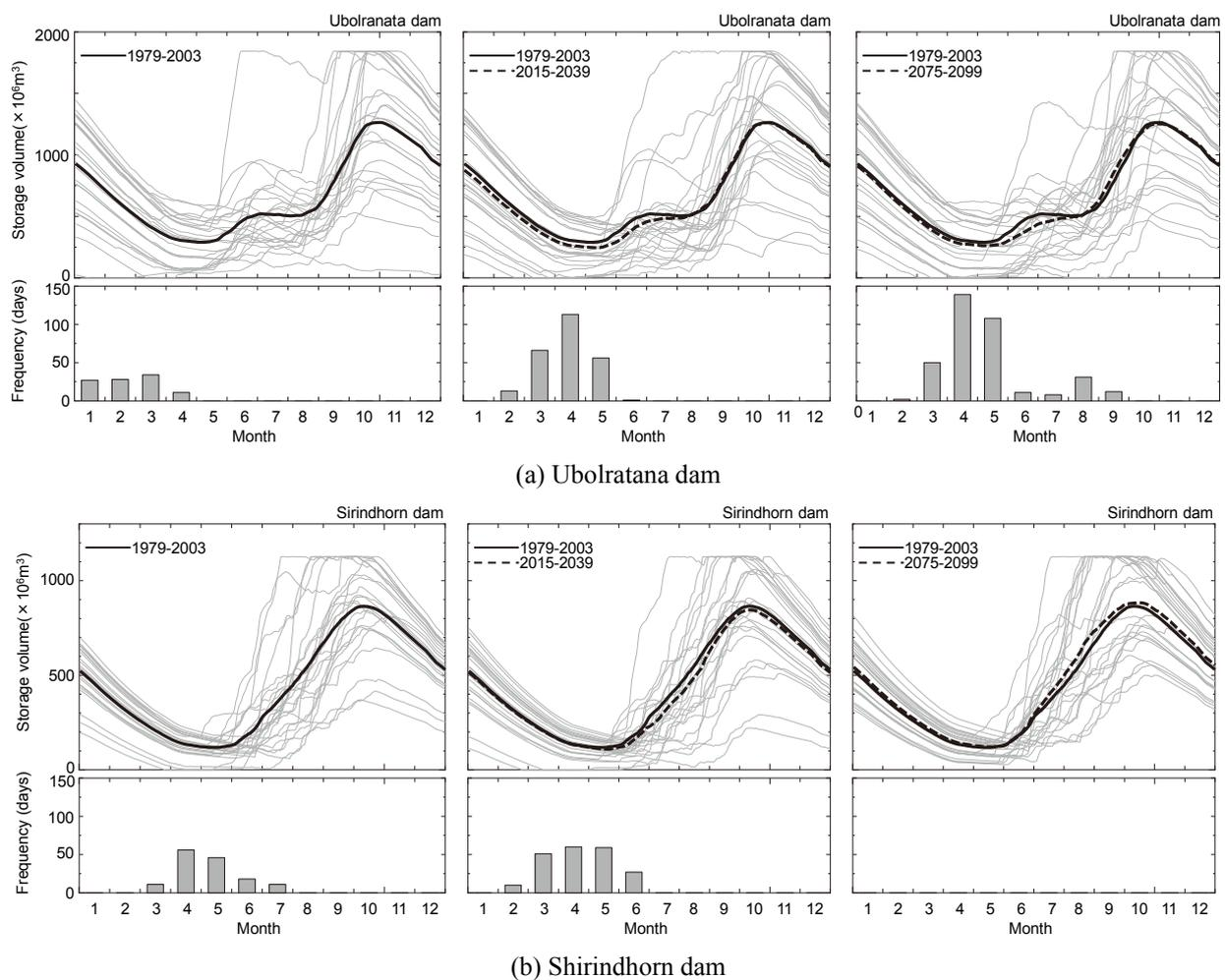
**Fig. 12.** Changes in storage volume and the frequency of empty days (no water storage) at the (a) Ubolratana and (b) Shirindhorn dams
