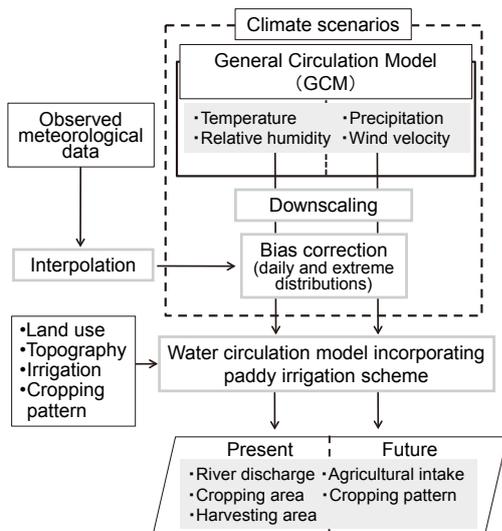
**Fig. 6. Procedure to assess climate change on water resources using a water circulation model and climate scenarios (Kudo et al. 2012)**
