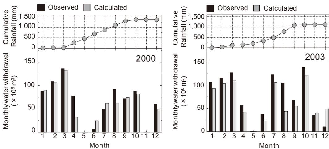
**Fig. 8. Comparison between actual and simulated amounts of monthly diversion water at the Nonwai weir in 2000 and 2003**
