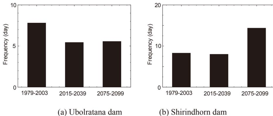
Fig. 13. Changes in the frequency of occurrence of daily spillway discharge (total days during 25 years) at the (a) Ubolratana and (b) Shirindhorn dams
