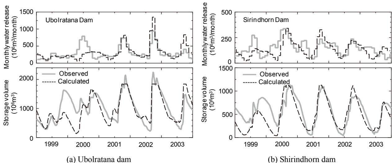
**Fig. 7. Simulation results of storage volume and water release at the Ubolratana and Shirindhorn dams**
