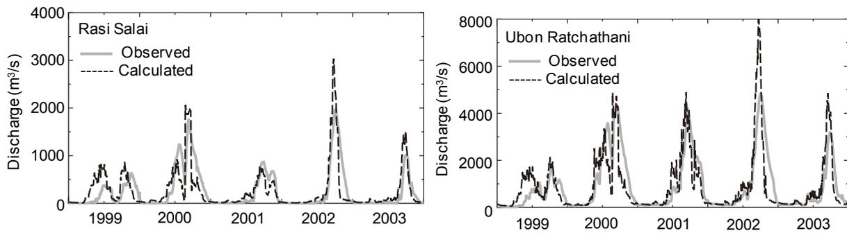
Fig. 9. Example simulation results of river discharges at the two hydrological stations
