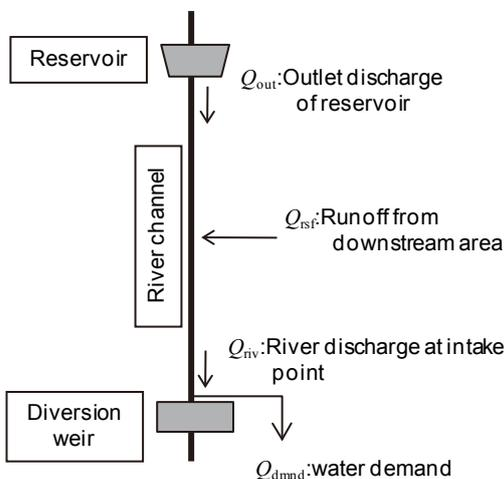
Fig. 4. Conceptual diagram of irrigation release by a reservoir operation model
