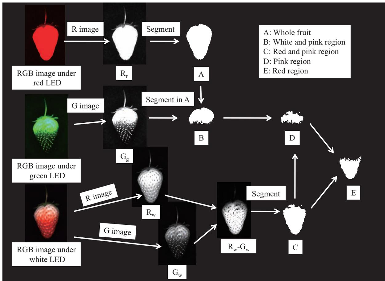
Fig. 8. Image and segmented region to measure coloration
