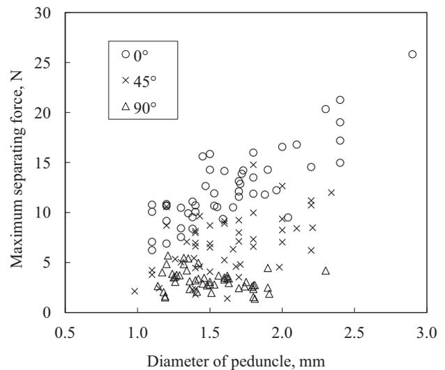
**Fig. 3. Plot of diameter of peduncle and maximum separating force with pulling angles of 0, 45, and 90°**
