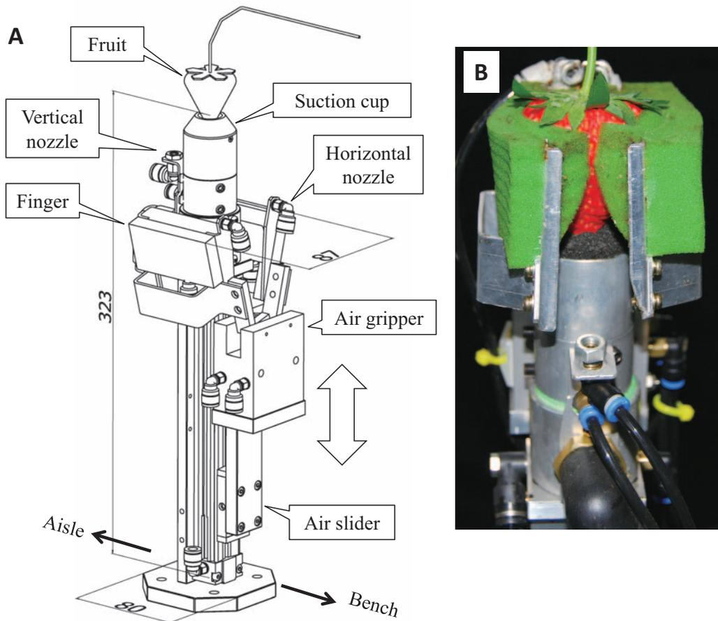
Fig. 9. Schematic diagram of the end-effector
