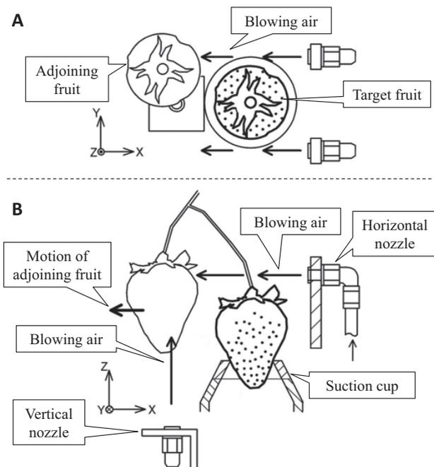
Fig. 10. Separation of adjoining fruit by blowing air
