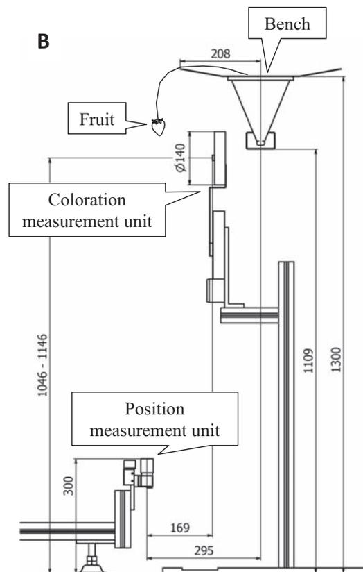
**Fig. 6. Schematic diagram of the machine-vision system**
