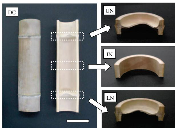
**Fig. 1. Upper node (UN), internode (IN) and lower node (LN) of a dead bamboo culm (DC) of *Phyllostachys pubescens***
