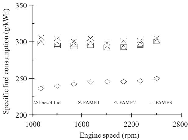
**Fig. 3. Relation of engine speed and specific fuel consumption**
