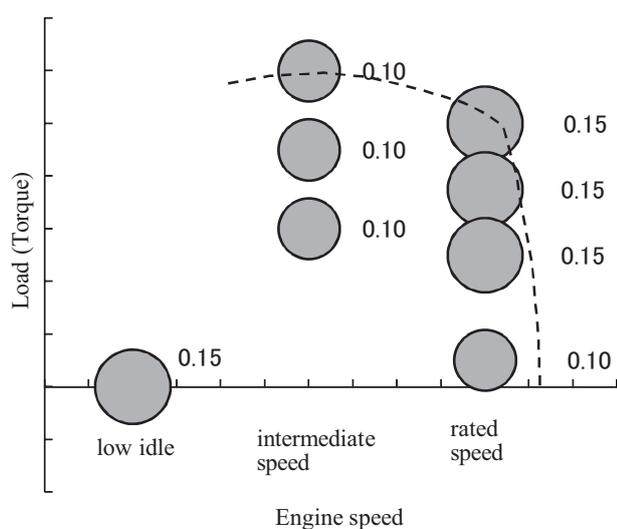
**Fig. 1. Measuring point and weighting factor of the 8mode test<sup>1</sup>**
