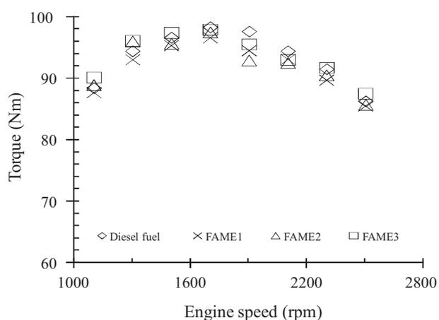
**Fig. 2. Relation of engine speed and torque**
