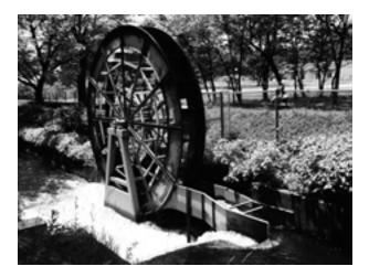
Fig. 3. A paddle (undershot) wheel (Tochigi Prefecture) Max. output: 1.8 kW; flow rate: 0.6 m<sup>3</sup>/s; diameter of wheel: 6 m.
