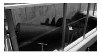
Fig. 5. An Archimedes wheel (Yamanashi Pref.) Max. output: 7.3 kW; max. flow rate: 0.99 m<sup>3</sup>/s; water head: around 1.0 m; length of wheel: 2.89 m; diameter: 1.6 m.
