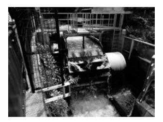
Fig. 6. An overshot wheel (Yamanashi Pref.) Max. output: 19 kW; max. flow rate: 0.99 m<sup>3</sup>/s; water head: around 3.5 m; diameter of wheel: 3 m.
