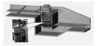
Fig. 7. Water turbine (Kaplan) installed at a drop along an open channel (Tochigi Pref.) Max. output: 30 kW; water head: around 2 m; max. flow rate: 2.4 m<sup>3</sup>/s.
