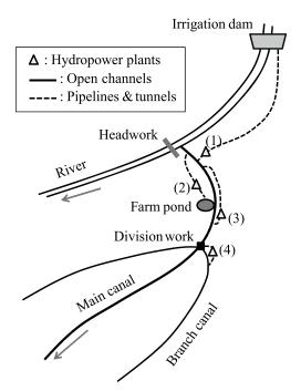
Fig. 1. Schematic diagram of possible hydropower generation sites in an irrigation canal system
