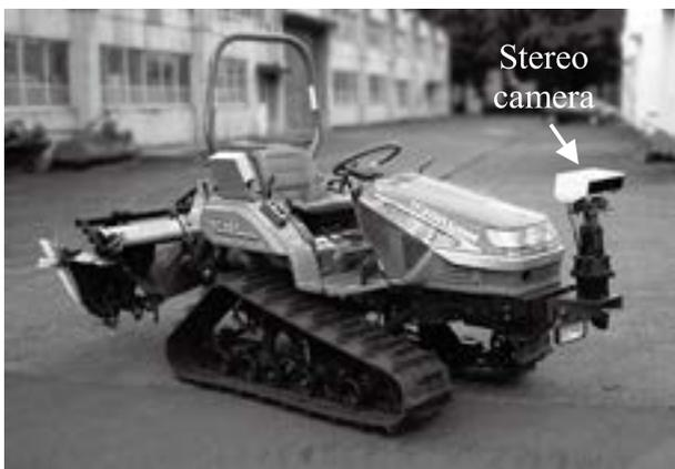
Fig. 1. Developed stereo camera mounted on the front of the tractor
