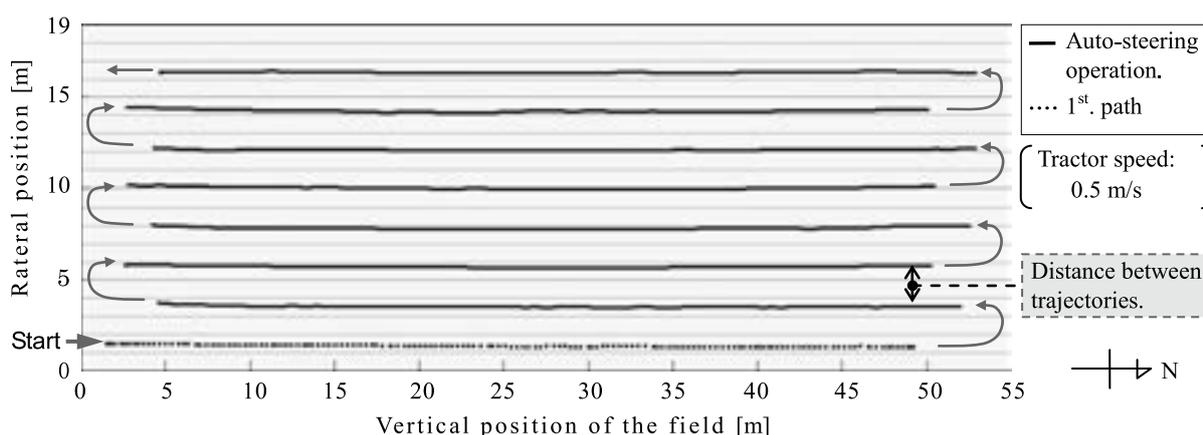
Fig. 12. Test result: trajectories of the tilling device edge
