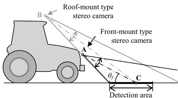
Fig. 3. Mounting location of the stereo camera and its viewing area
