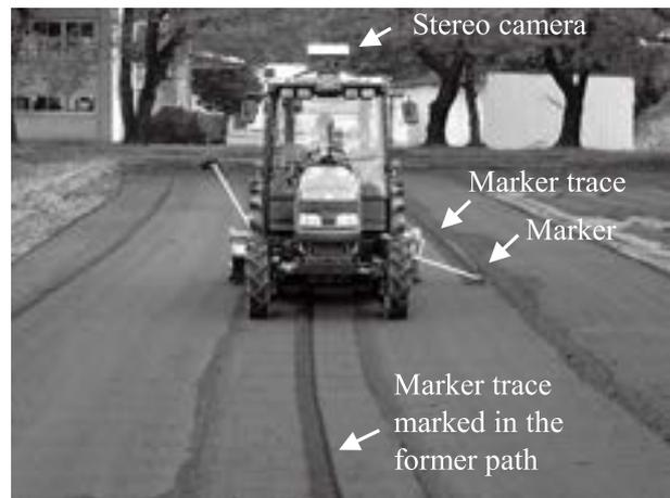
Fig. 2. Roof-mounted stereo camera, engaged in tracking a marker trace
