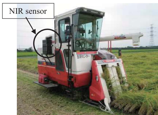
Fig. 5. Developed NIR sensor mounted on the yield monitor combine
