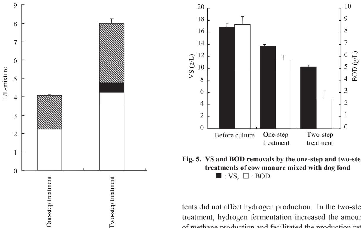
**Fig. 4. Total biogas production by the one-step and two-step treatments from cow manure mixed with dog food**
