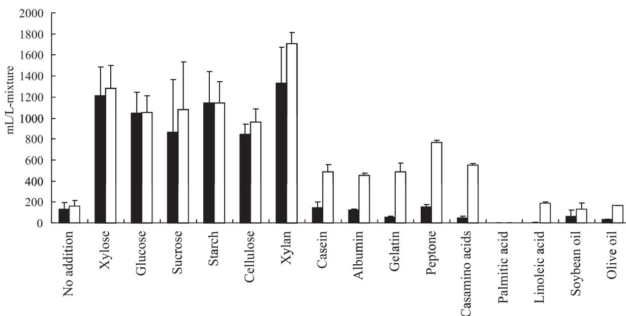
Fig. 1. Hydrogen production from cow manure mixed with defined substrates
