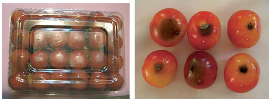
Fig. 7. Damage to packaged cherries after transport from Yamagata to Taipei
