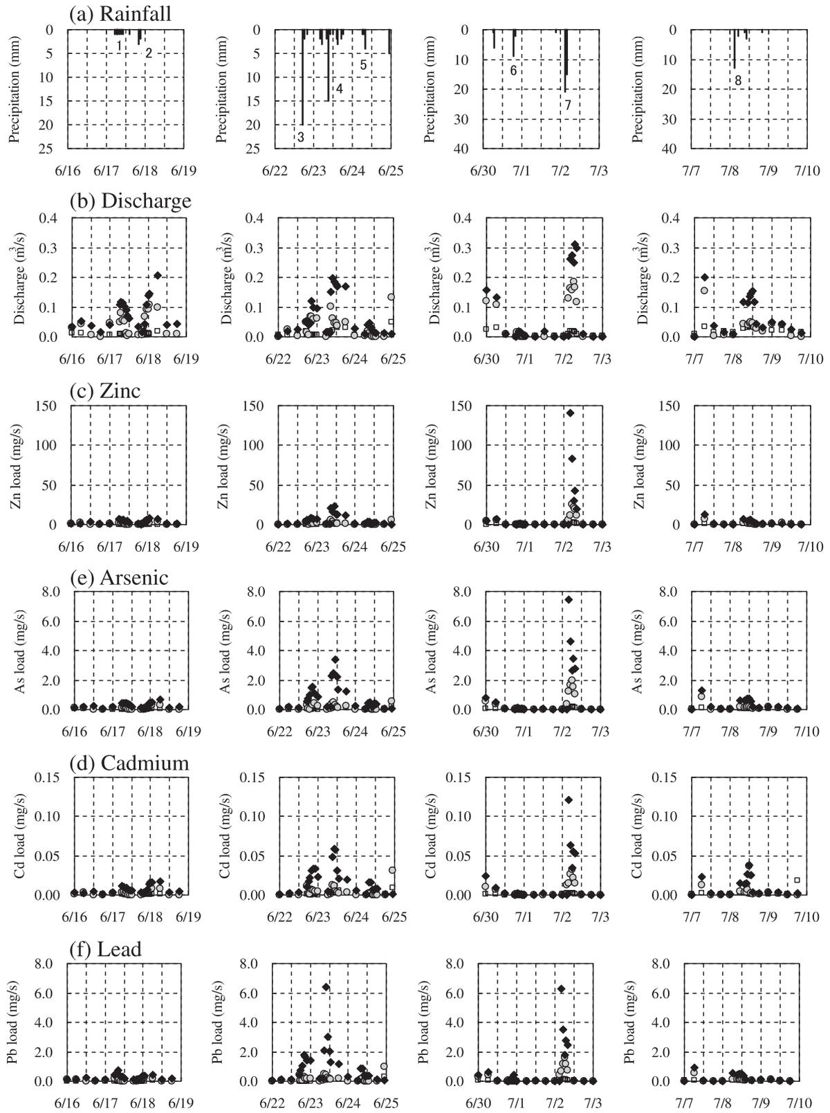
Fig. 4. Fluctuation of discharge and heavy metal loads in the drainage canal
