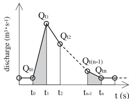
Fig. 2. Calculation method for the discharge during the rainfall events
