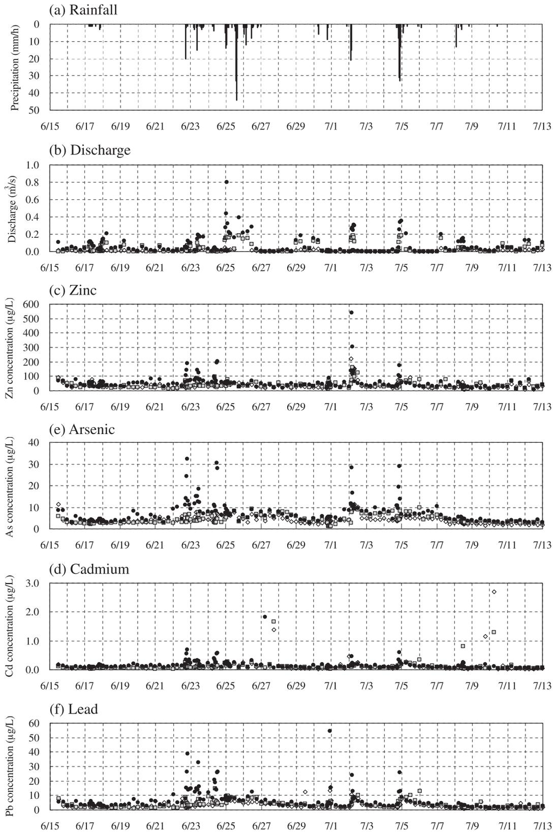
Fig. 3. Fluctuation of discharge and heavy metal concentrations in the drainage canal
