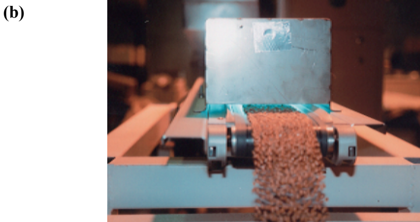
Fig. 1. Schematic diagram of recirculating grain sterilization equipment using ultraviolet irradiation a: Recirculation grain sterilization equipment using ultraviolet irradiation. b: View of UV irradiation for wheat.
