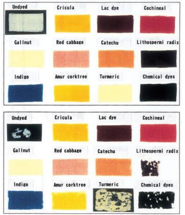
Fig. 2. Damage to wool fabrics dyed with natural dyestuffs by *Anthrenus verbasci* larvae 4 weeks after the beginning of the feeding test
