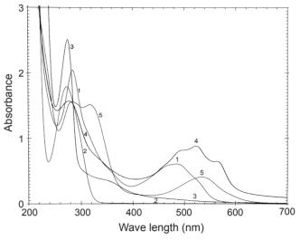
Fig. 5. Absorption spectra of natural dyestuffs – (1) 1: lac dye, 2: gallnut, 3: catechu, 4: Lithospermi radix, 5: red cabbage.
