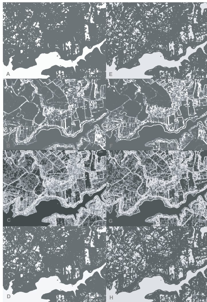
Fig. 5. Textural features derived from a 256 gray level image (A, B, C, D) and segmented image in 8 classes (E, F, G, H) with window size of 3 \times 3
