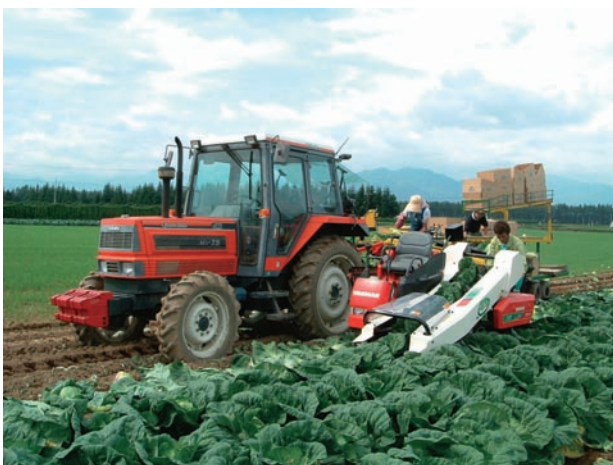
Fig. 4. Harvesting, processing, boxing and loading unified in one harvesting system
