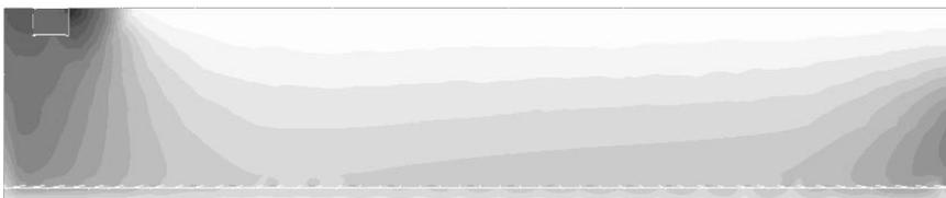
**Fig. 9. CFD computed relative humidity at the plane bisecting chimney A**
