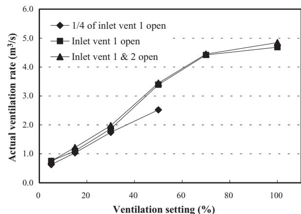
Fig. 6. Airflow rates through the chimney in the piglet house according to the fan ventilation setting
