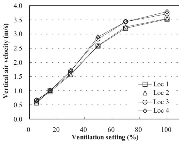
**Fig. 7. Vertical downward air velocities measured at the holes of the perforated ceiling for inlet vent 1 open (a) and inlet vents 1 and 2 open (b)**
