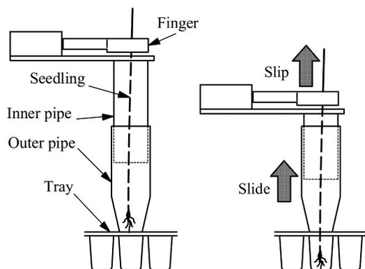
Fig. 4. Planting mechanism
