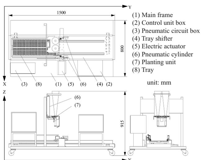
Fig. 6. Construction of planting machine
