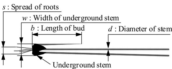
Fig. 2. Measured dimensions of seedling
