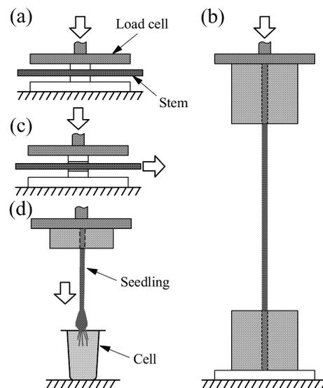
Fig. 3. Measuring methods for mechanical properties of seedling
