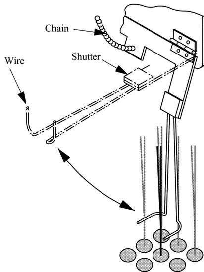
Fig. 12. Mechanism to secure the seedling path
