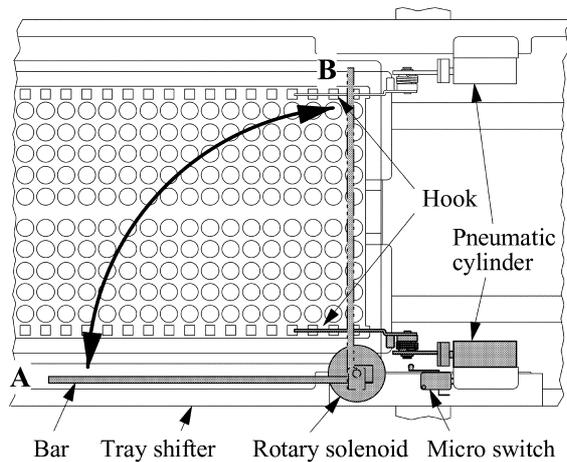
Fig. 11. Mechanism to arrange posture of seedlings
