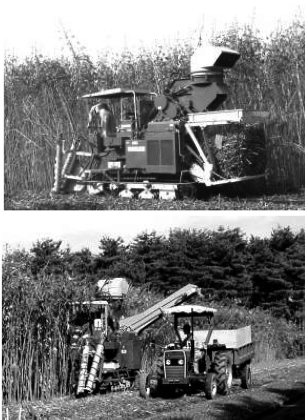
Fig. 1. Operation of the kenaf harvester Upper, net bag type; bottom, conveyor type.
