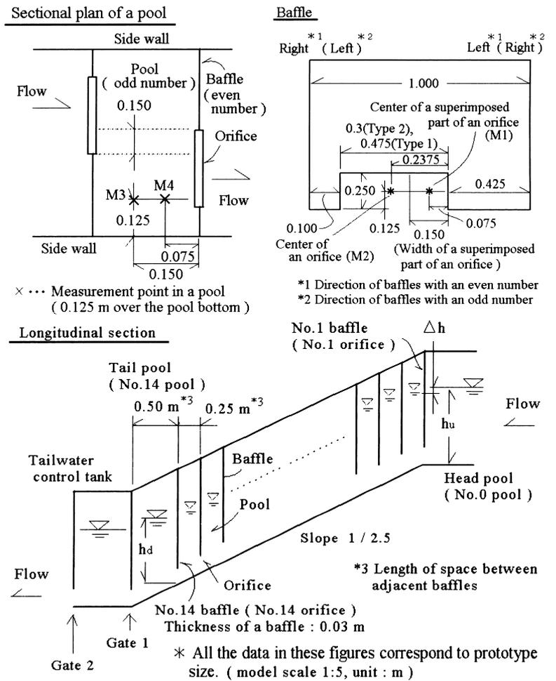
Fig. 4. Whole model of a submerged orifice fishway
