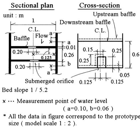
Fig. 3. Partial model of a submerged orifice fishway
