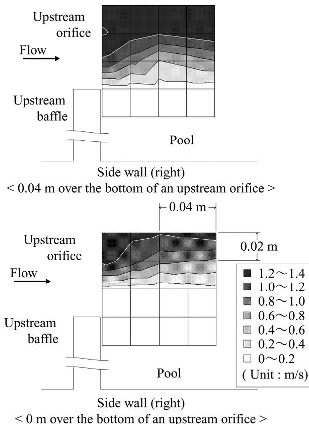
**Fig. 5.  $(V_{xyz})_{av}$  contours downstream of the upstream orifice in the partial model**
