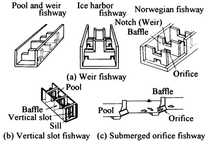
Fig. 1. Classification of artificial fishways (pool type)
