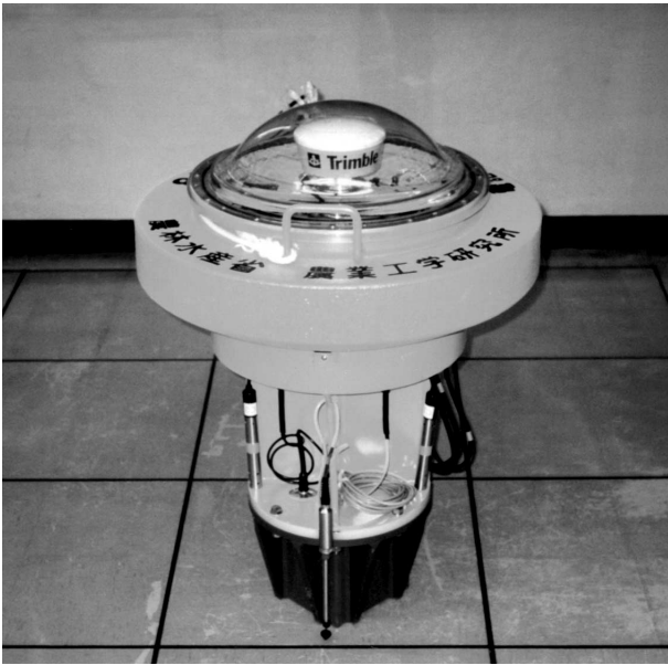
Fig. 1. Drift type buoy developed for the observation of current and water quality
