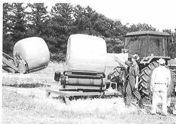
Fig. 3 Wrapping of cereal straw with plastic stretch film
