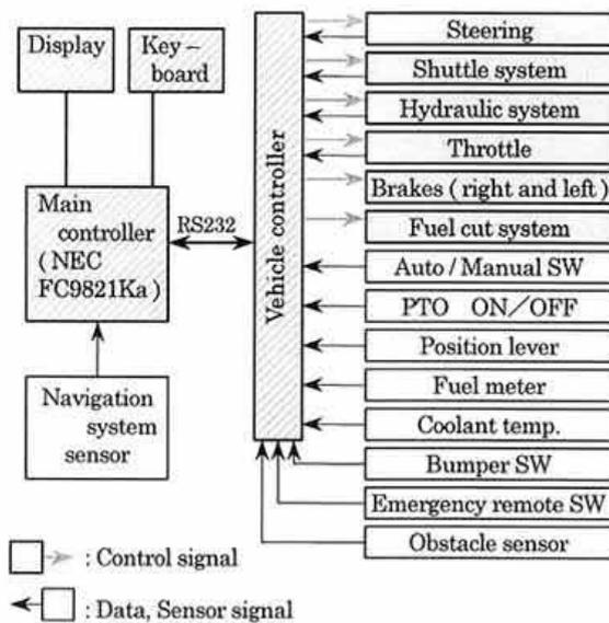
Fig. 4. Control systems of the ROBOTRA
