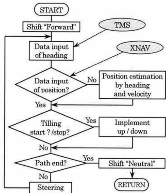
Fig. 7. Flow chart of straight operation routine
