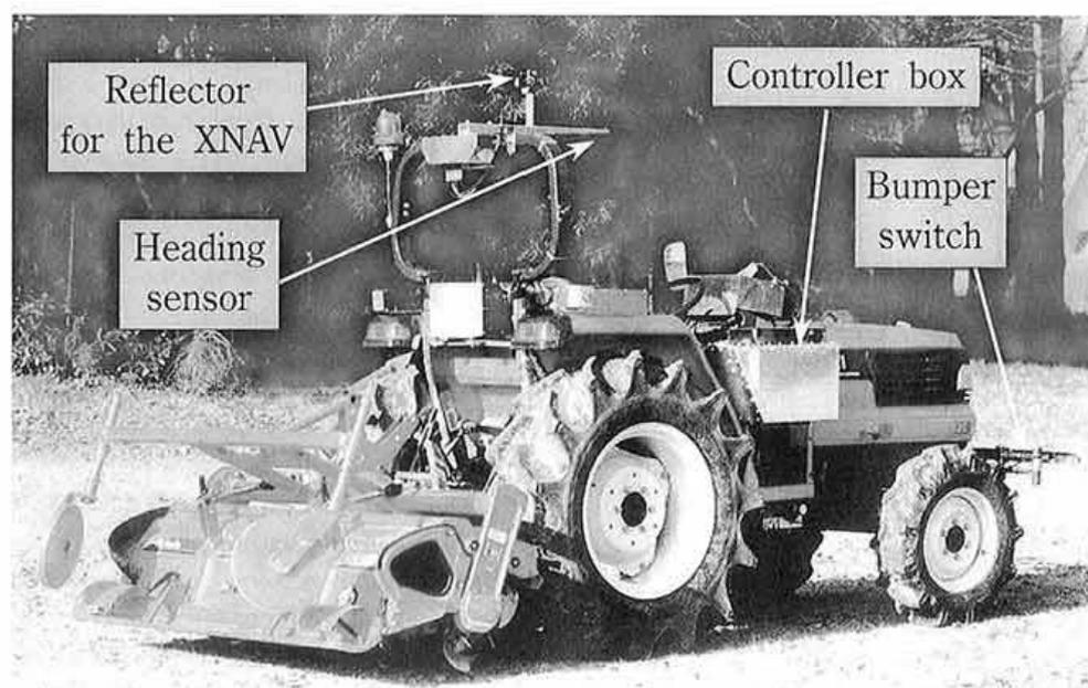
**Fig. 3. Robotized vehicle "ROBOTRA"**
