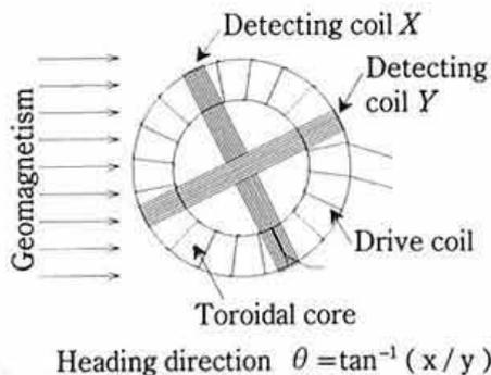
**Fig. 1. Principle of measurement of geomagnetic sensor**
