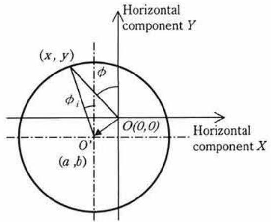
**Fig. 2. Influence and calibration of magnetic environment**
