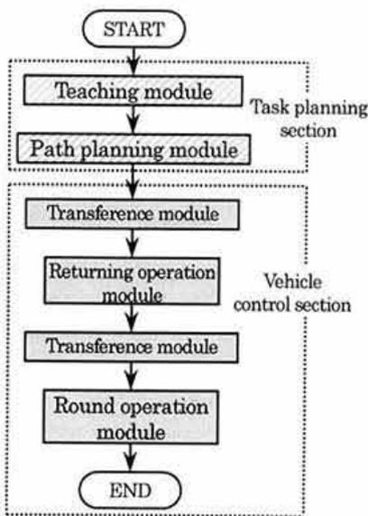
Fig. 6. Main flow chart of operation
