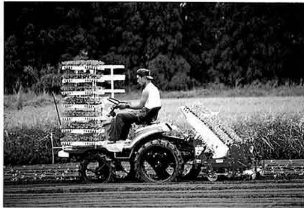
Fig. 8. Fully automatic transplanter model SKP20 for cell mold seedlings (Kubota, Co., Ltd., used in Takeda, Kumamoto)
