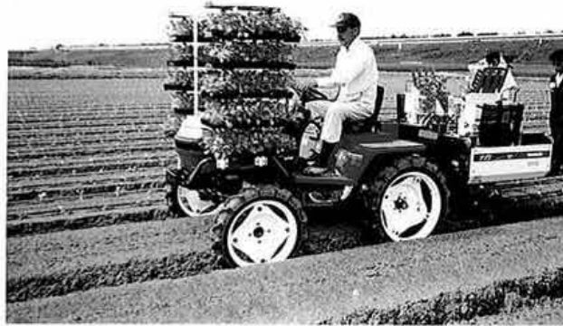
Fig. 7. Fully automatic transplanter Model PR2 for cell mold seedlings (Yanmer Noki, Co., Ltd, for cabbage in Ogoori, Fukuoka)
