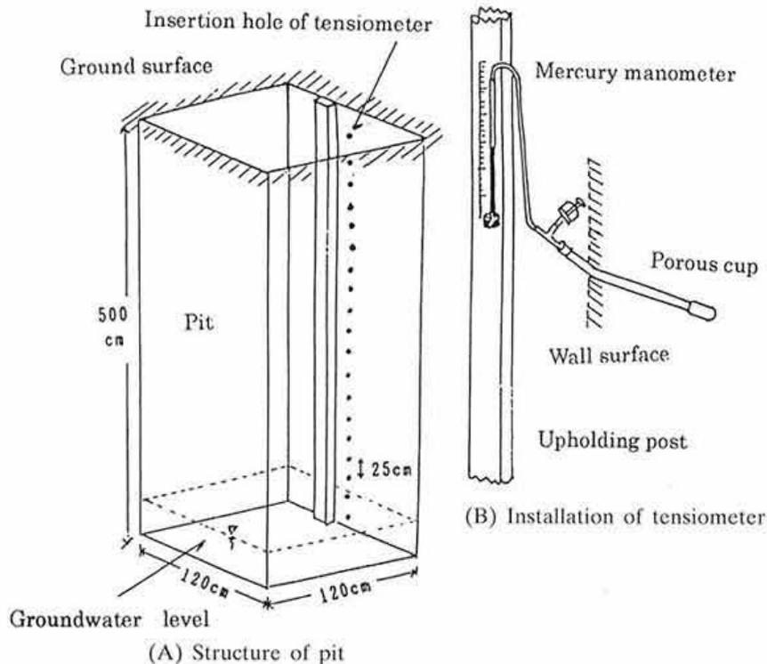
Fig. 3. Method of measurement of soil moisture content<sup>2)</sup>
