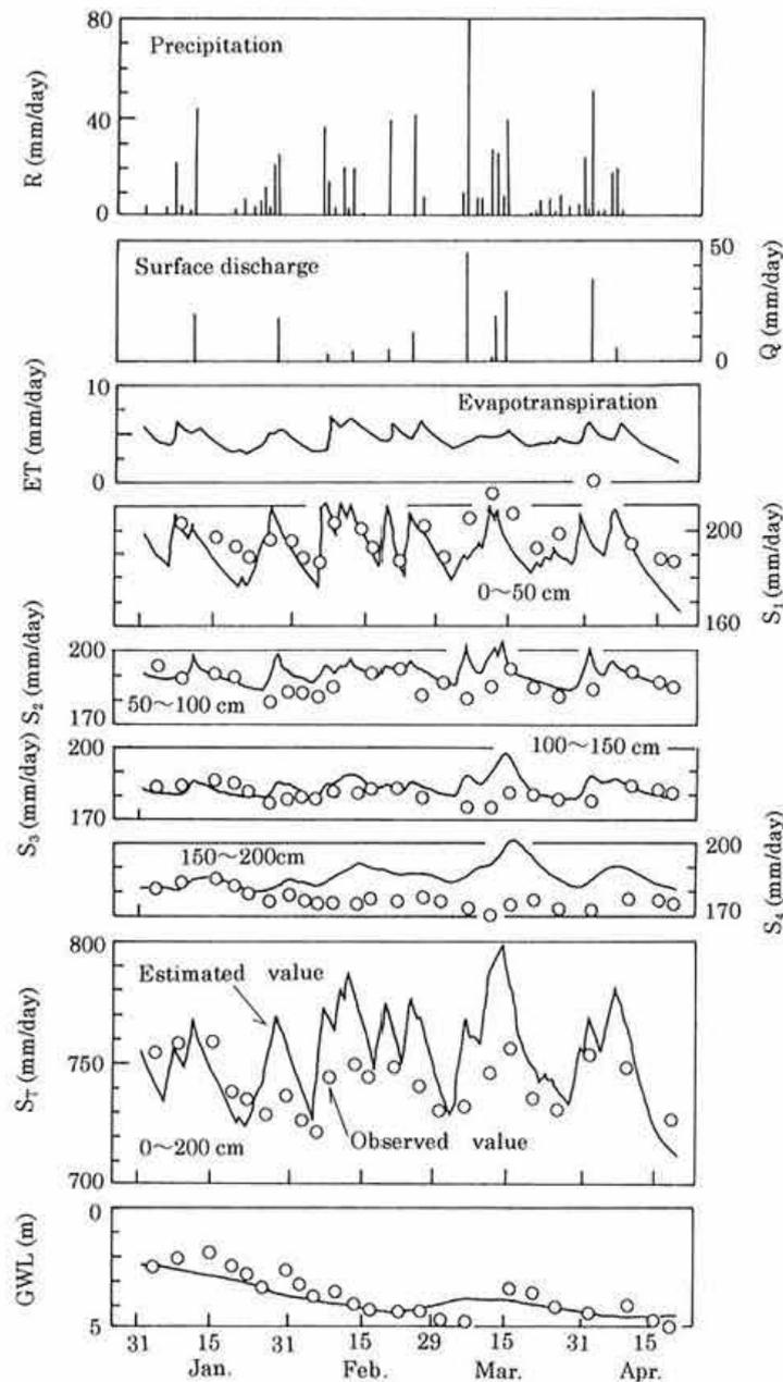
**Fig. 6. Comparison of estimated values of soil moisture, groundwater level and evapotranspiration at Pit 2 with observed values**
