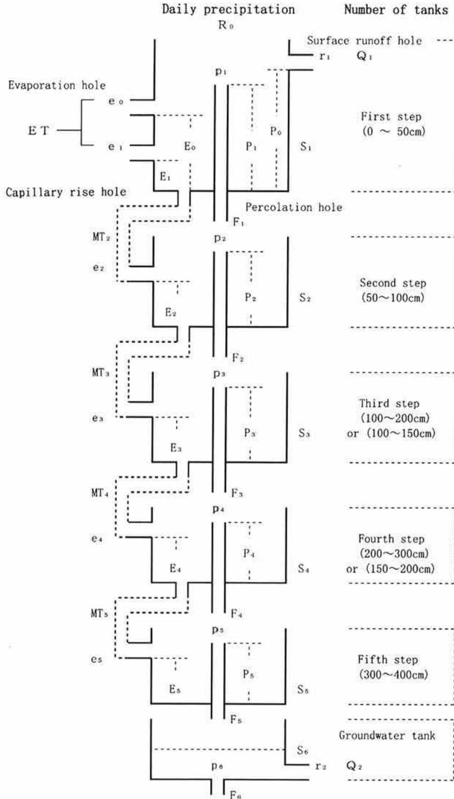
Fig. 1. Schematic illustration of the TANK-model
