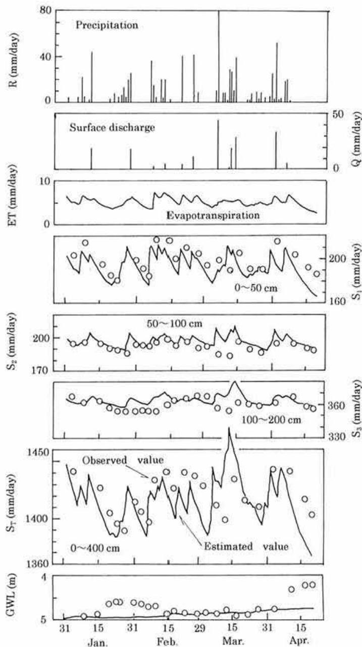
Fig. 5. Comparison of estimated values of soil moisture, groundwater level and evapotranspiration at Pit 1 with observed values
