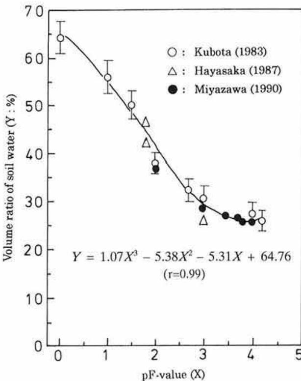
Fig. 4. Curve of moisture characteristics of Cerrados soils
