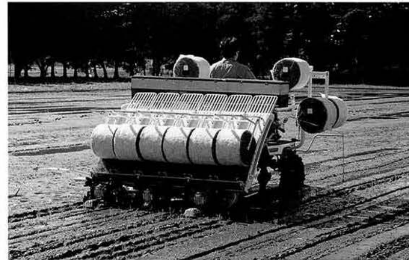
Fig. 10. Rice transplanter for roll type seedlings
