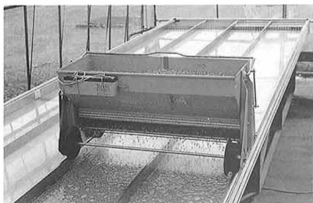
Fig. 2. Nursery device and self-propelled seeder
