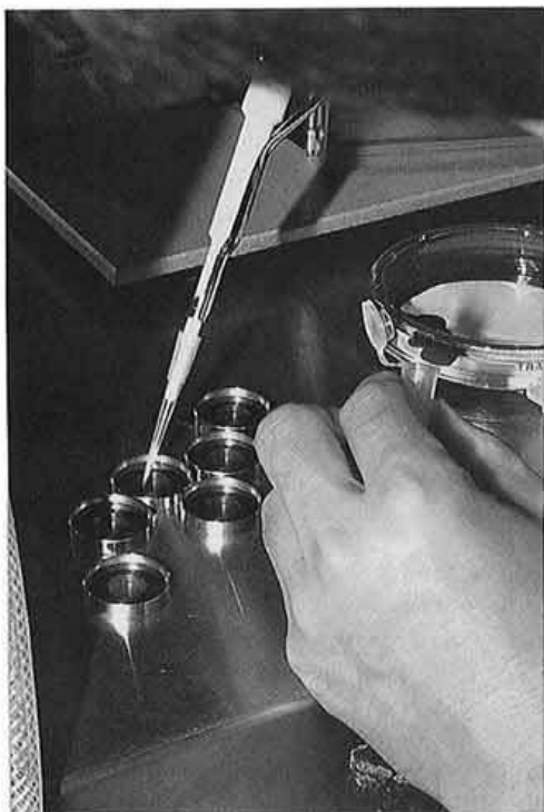
Fig. 6. Coating microcarriers (DNA-coated particles) over a macrocarrier
