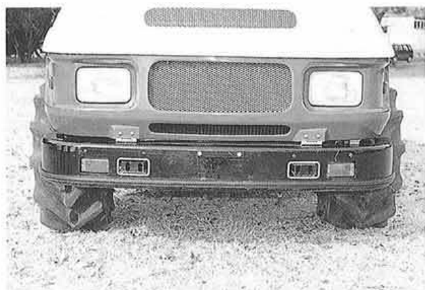
Fig. 7. Ultrasonic sensors and touch sensor
