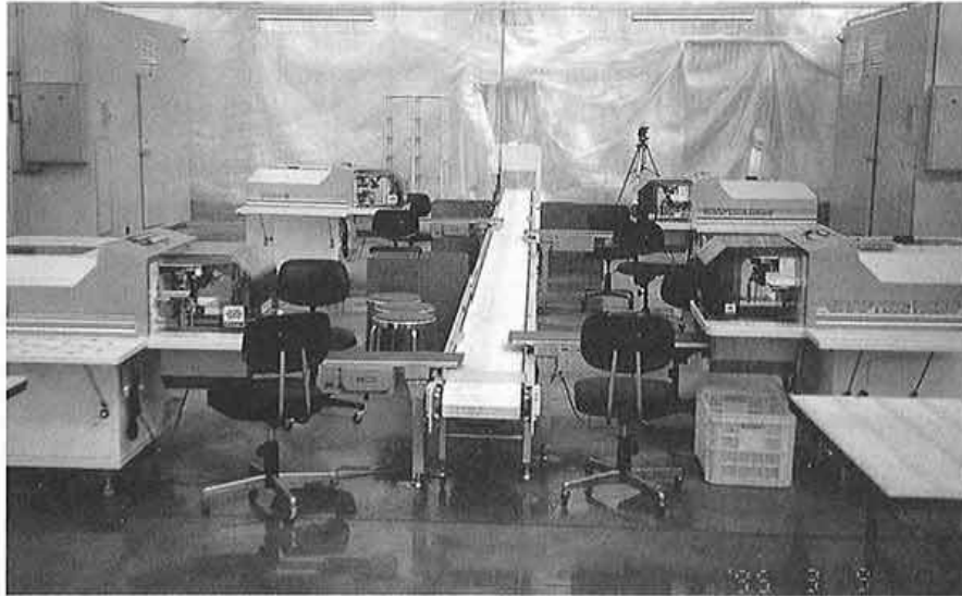
Plate 4. Grafting systems introduced in a seedling production plant Four systems are arranged on both sides of the belt conveyor. Artificial acclimation systems are seen on both sides.
