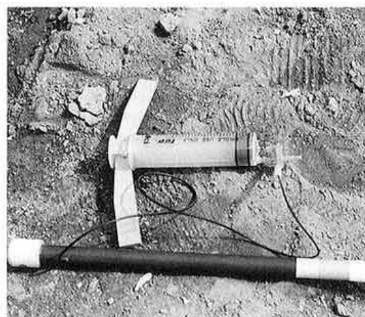
Plate 1. Tool for the collection of the soil solution
