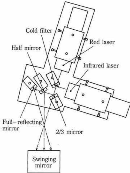
Fig. 4. Optical arrangement
