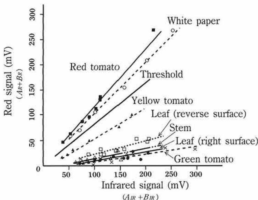
Fig. 7. Relationship between infrared and red signals
