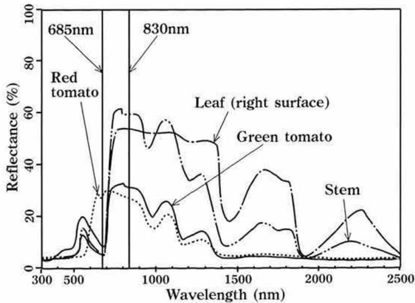
Fig. 2. Reflectance characteristics of tomato plant
