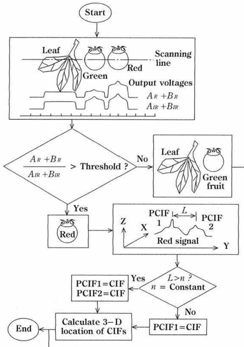
Fig. 10. Flow chart of signal processing
