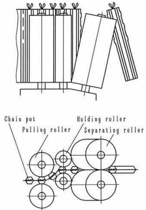
Fig. 2. Structure of separating mechanism
