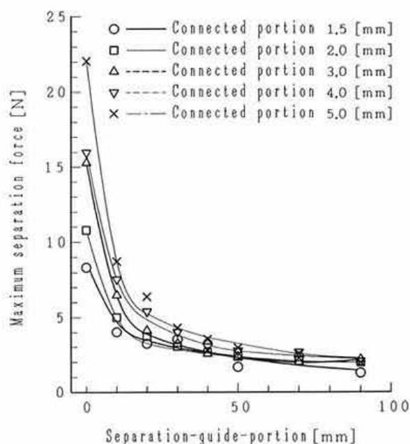
Fig. 5. Relationship between the separation force and the length of the separation-guide-portion
