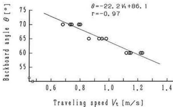
Fig. 8. Relationship between traveling speed and the value of the backboard angle
