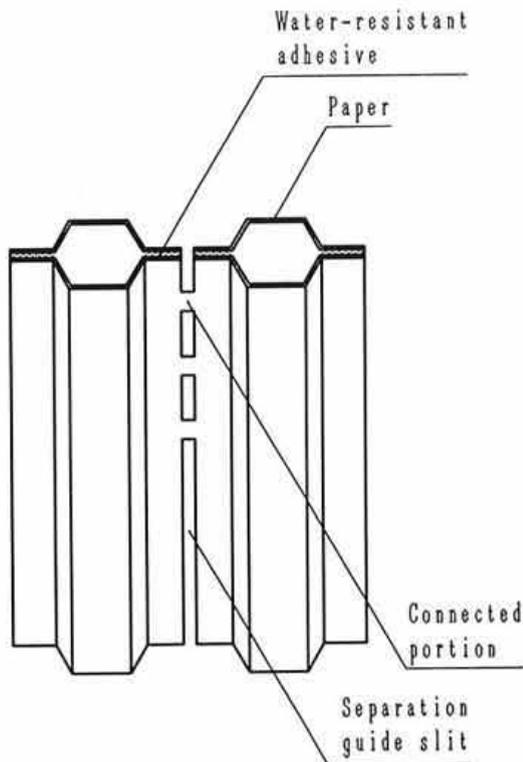
Fig. 1. Structure of chain pots
