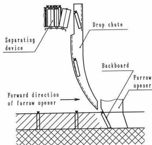
Fig. 4. Transplanting mechanism of the new drop chute type
