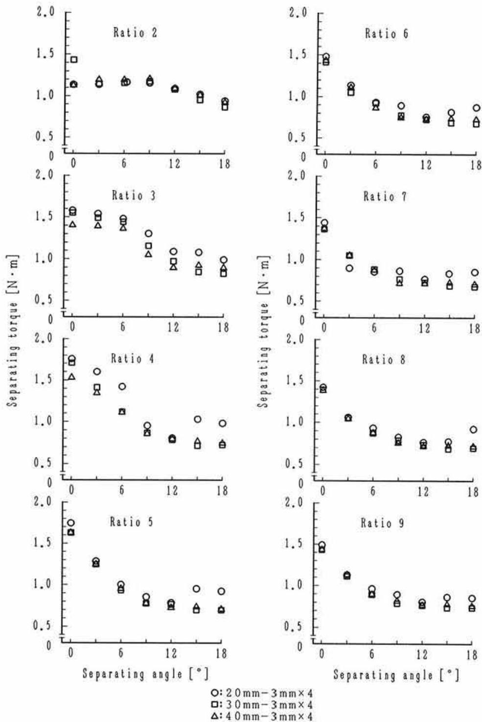
Fig. 6. Relationship between the separating angle and separating torque
