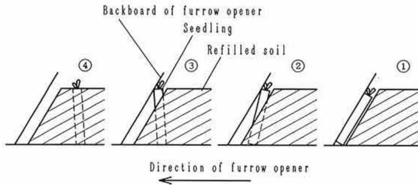
Fig. 7. Schematic representation of seedlings held in soil by the furrow opener
