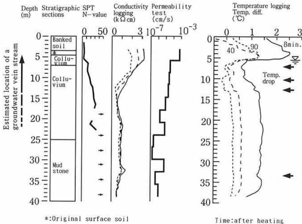
Fig. 7. Profile and results of tests from boring hole B3
