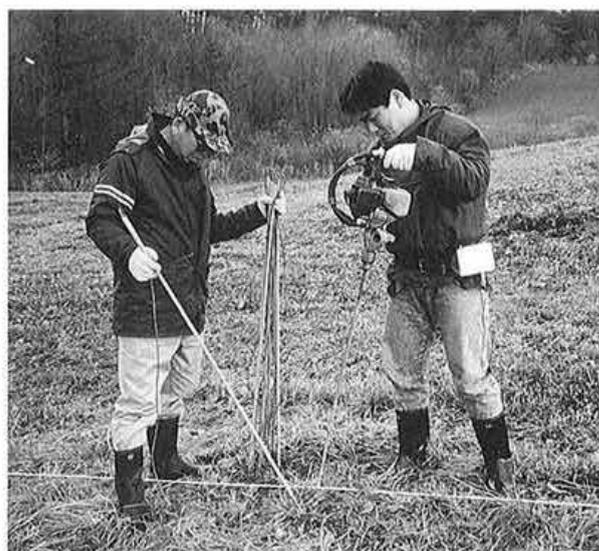
Plate 1. Motor-driven auger used for the drilling of a measurement hole
