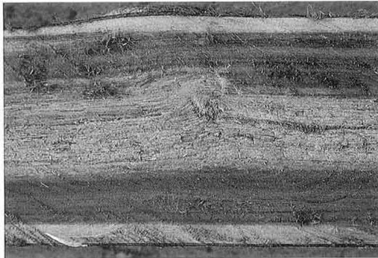
Plate 2. Advanced decay (disease index R_4 )
