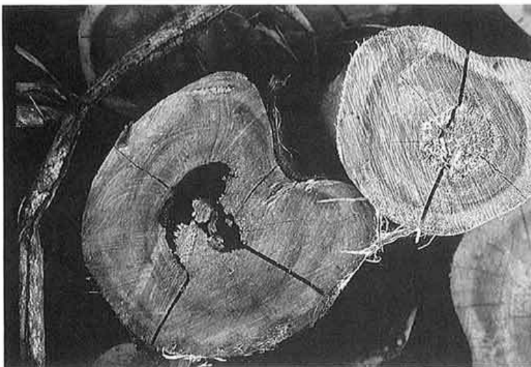
Plate 3. Hollow in heartwood due to heart rot
