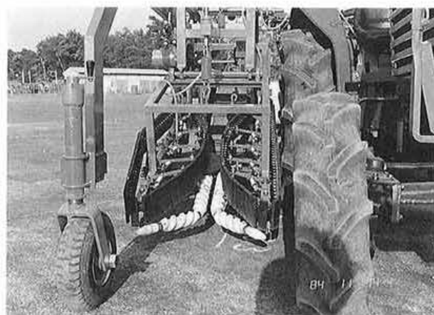
Plate 3. Front view of screw augers and feed belts
