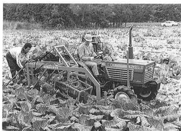
Plate 2. Lateral view of tractor-mounted-type harvester
