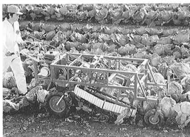
Plate 1. Lateral view of walking-type harvester
