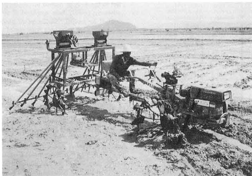
Plate 1. Seeding operation with the 12-row drill seeder under wet soil conditions
