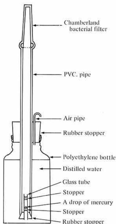
Fig. 5. Structure of the Okanoué's evaporimeter
