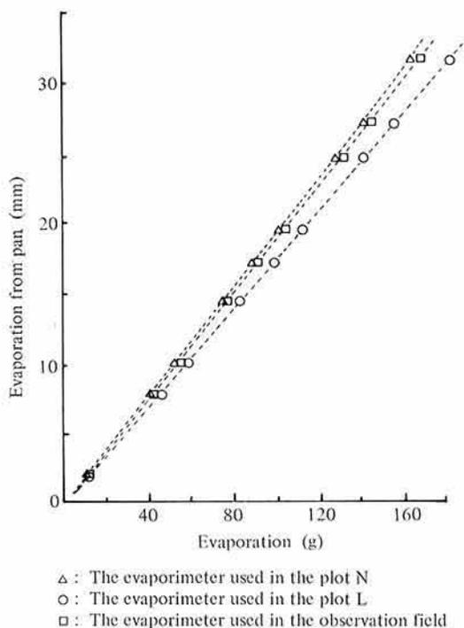
Fig. 6. Relationship between evaporation from the pan and that from the Okanoué's evaporimeter
