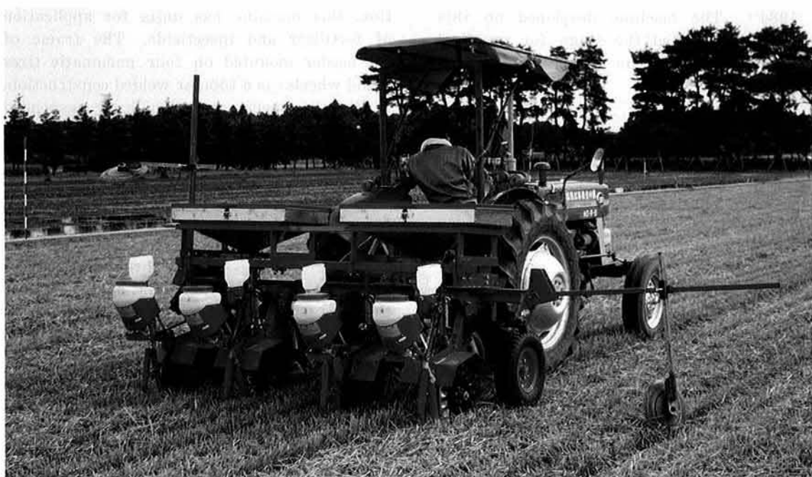
Plate 1. The newly developed no-till seeder in operation
