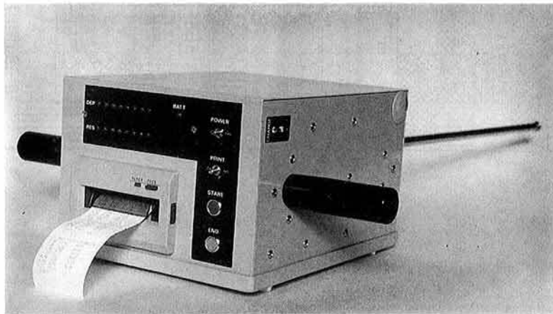
Plate 1. Simple type computer-aided cone-penetrometer with one-man operation.
