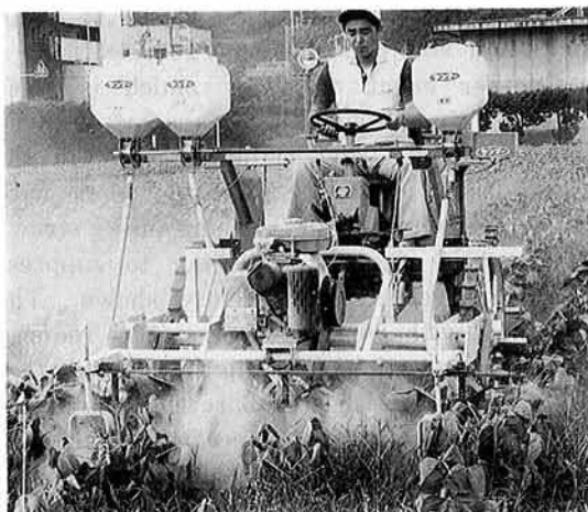
Plate 2. Intertillage and ridging with the riding type multiple-row crop-management machine
