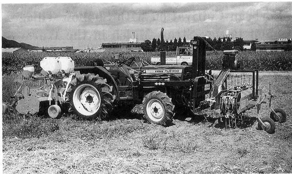
Plate 1. The newly developed machine for shallow tillage and straw mulching, composed of a belt type rake, a rotary planter, and a herbicide duster, mounted on a tractor
