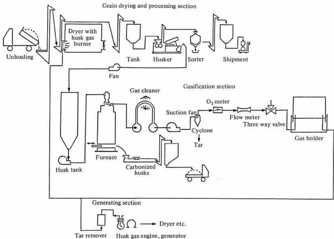
Fig. 3. Flow chart of the pyrolytic gasification system for rice husks
