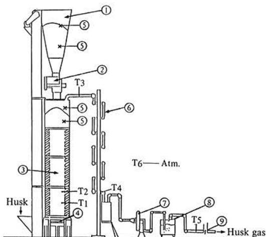
Fig. 1. Schematic figure of the pyrolytic gasification system for rice husks (DHF791 and 801 type)
