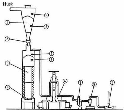
Fig. 2. Schematic figure of the pyrolytic gasification system for rice husks (DHF821 type)
