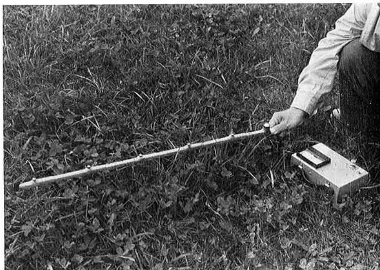
Plate 1. External appearance of the portable solarimeter newly devised by the author and his co-workers
