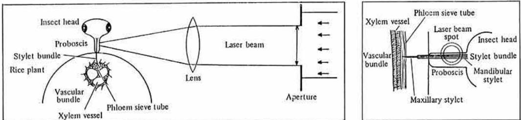
1. Diagrammatic representation of a cross section of the rice plant, the insect head, and YAG laser beam focused on proboscis for stylectomy.
