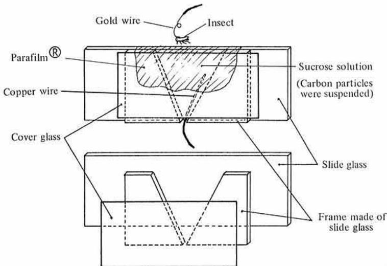
Fig. 4. Observation chamber which is built easily
