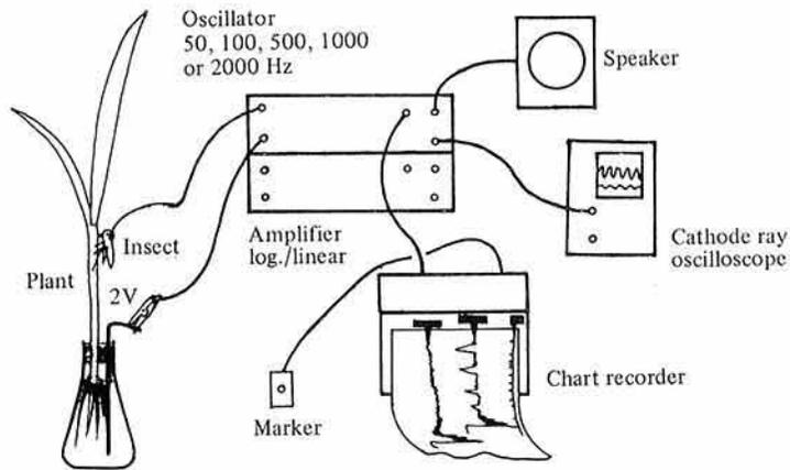
Fig. 3. A diagrammatic representation of the improved system of EMIF and a leafhopper probing a rice plant, showing the points of attachment to the system
