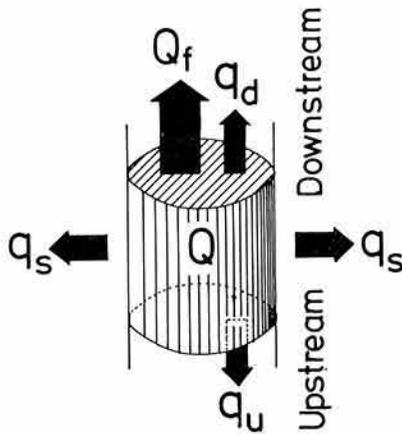
Fig. 1. Heat balance for a stem segment to which energy,  $Q$ , is supplied
