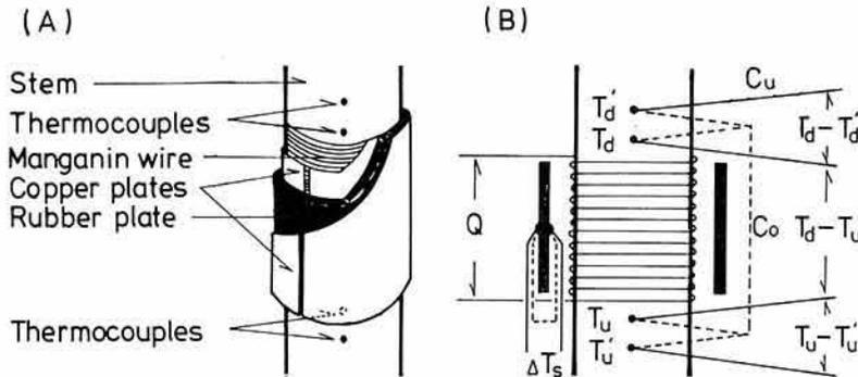
Fig. 2. Apparatus for measuring the water flow rate in plant stem (A) and its setup (B)
