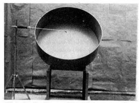
Plate 1. Coating machine (Rotary pan with a separate attachment for water spray)
