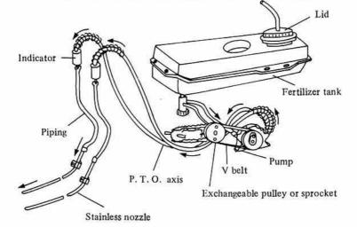
Fig. 2. Applicator for paste-like fertilizer
