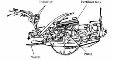
Fig. 1. Rice seedling transplanter equipped with an applicator for simultaneous application of paste-like fertilizer
