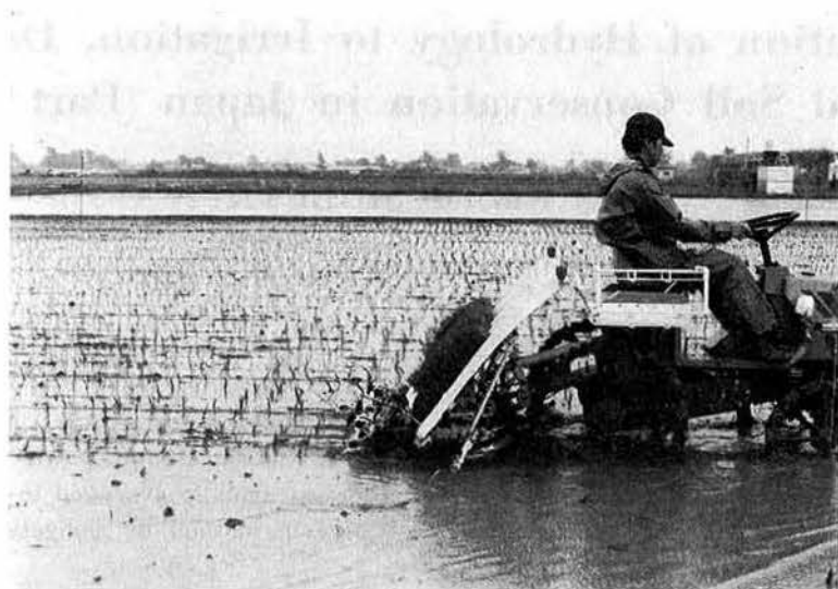
Plate 1. Field performance test of riding type rice transplanter
