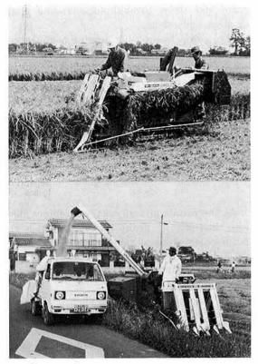
Plate 1. Combine harvester used in Japan
