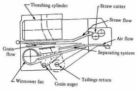
Fig. 2. Cross-section of the threshing device of combine harvester
