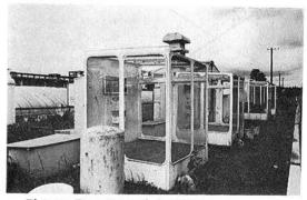
Plate 2. Experimental facility to measure plant growth and dry matter production under natural light with chronic exposure to SO<sub>2</sub> gas.
