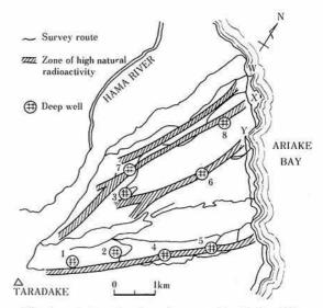
Fig. 1. Areas showing strong radioactivity (W, X, Y and Z zones) identified by the survey using a car-mounted groundwater-prospecting instrument
