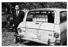
Plate 1. Car-mounted groundwater-prospecting instrument
